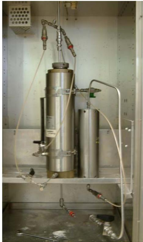
Fig. B1 - Core Leak-Off Test Apparatus.
