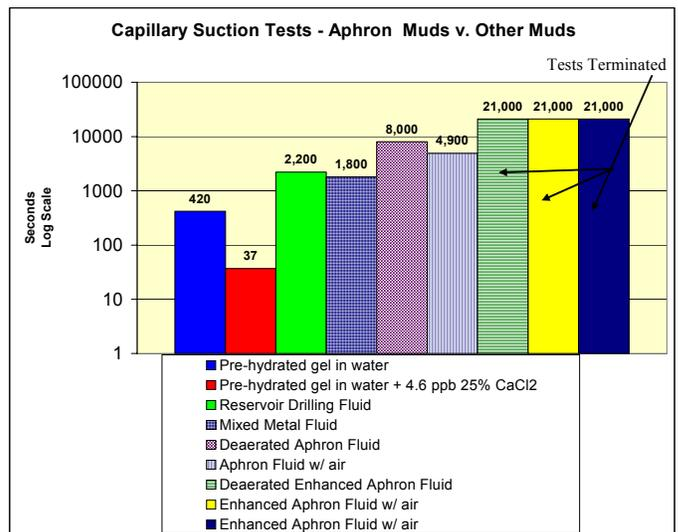
Fig. 1 - CST Results - Standard CST Procedure.
