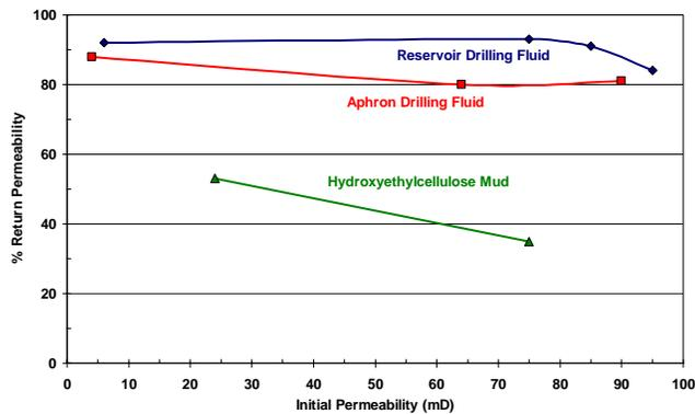
**Fig. 13 – Aphron drilling fluids yield similar return permeabilities as high-performance reservoir drilling fluids. [Tests conditions: Berea sandstone, 150 °F,  $P_{inlet}=2500$  psig,  $P_{outlet}=2000$  psig,  $P_{confining}=3000$  psig]**
