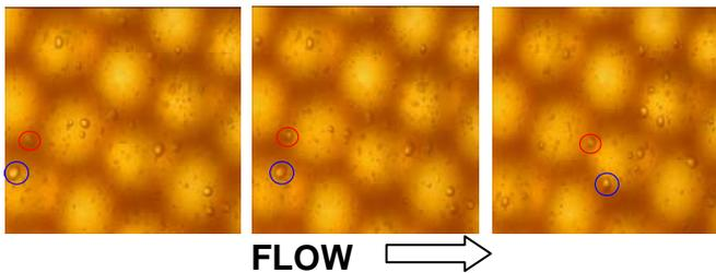
**Fig. 5 – Velocity of aphrons increases with increasing size. The bubble in the blue circle is about 25% larger than the one in the red circle.**
