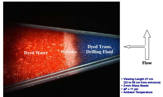
**Fig. 6 - Bubbly flow of aphrons produces a band of bubbles of constant thickness at the interface between the drilling fluid and the reservoir fluid.**
