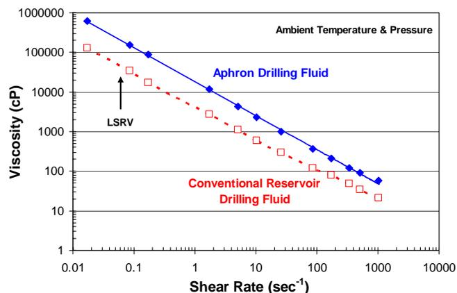
**Fig. 11** – Aphron drilling fluids are power-law fluids, like conventional reservoir drilling fluids, but they possess significantly higher LSRV.
