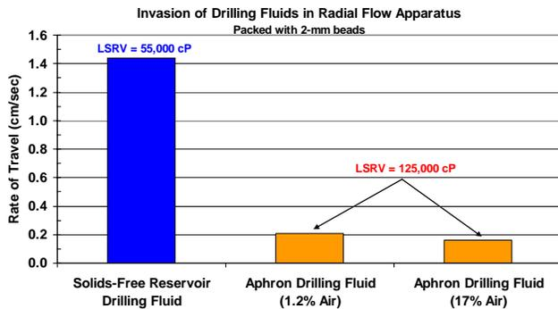
**Fig. 12 – Aphron drilling fluids control fluid invasion into a packed bed significantly better than conventional reservoir drilling fluids.**
