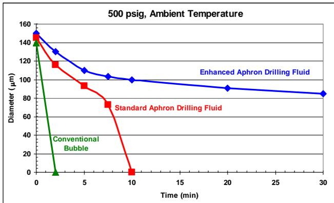
**Fig. 3 – Aphrons withstand elevated pressures much better than do conventional bubbles**
