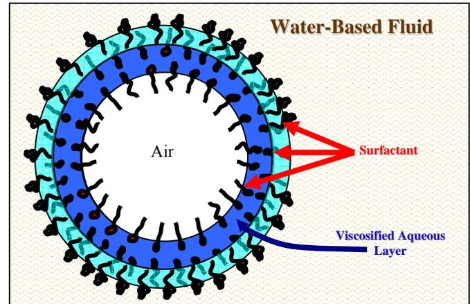
**Fig. 2 – Schematic of an aphron (after Sebba<sup>2</sup>)**
