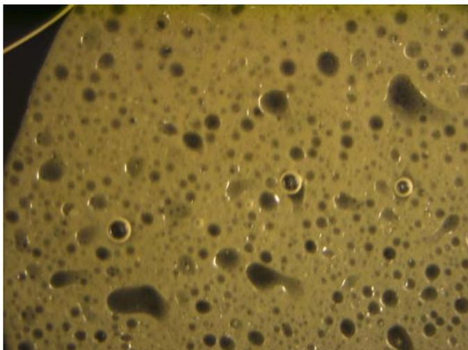
**Fig. 9** – Microscopic examination of 50/50 dispersion of a crude oil and an aphron drilling fluid. Spheres are aphrons, while the dark, less-well-defined structures are oil droplets.
