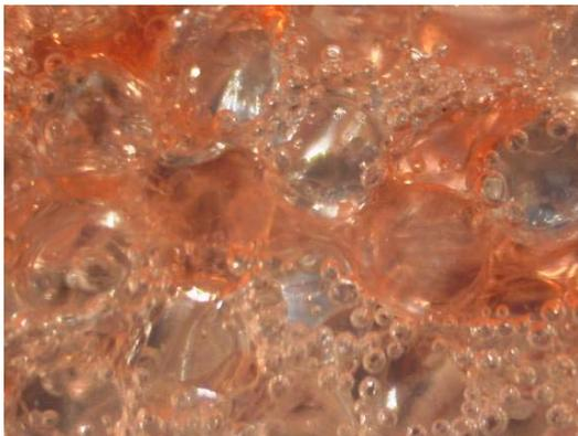
**Fig. 14 – Channeling of a produced oil (red liquid) through transparent aphron drilling fluid (colorless liquid containing bubbles) in a packed bed of 2-mm glass beads.**
