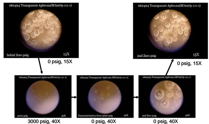
**Fig. 4 – Rapid Pressure Cycling of Aphron Drilling Fluids Leaves Most Aphrons Intact**
