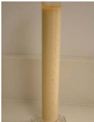
**Fig. 8** – Dispersion of 50 vol % each of a crude oil and an aphron drilling fluid.
