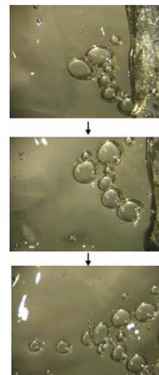
**Fig. 7 - Aphrons do not stick to each other or to the walls of pores and fractures.**
