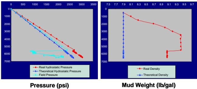
**Fig. 1 – RFT Log of Aphron Drilling Fluid used to drill in South American field**
