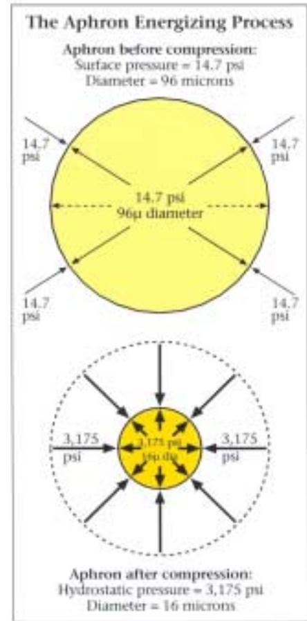
Fig. 4 – The aphron energizing process
