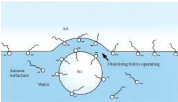
Fig. 2 – Structure of standard foam<sup>1</sup>
