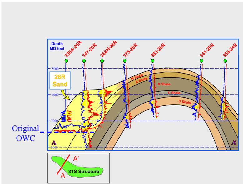
Fig. 7 – The 26R Miocene sands are steeply dipping turbidite sandstone reservoirs.
