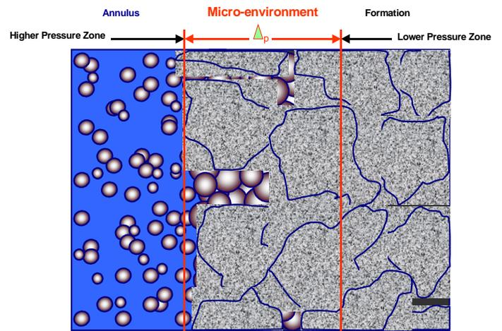
Fig. 5 – When the bit enters a low-pressure zone, the energized aphrons aggregate instantaneously within the formation, creating a micro-environment bridge, preventing invasion of whole drilling fluid, filtrate and solids
