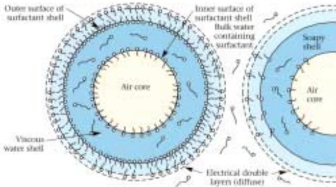
Fig. 1 – Structure of colloidal gas aphron<sup>1</sup>
