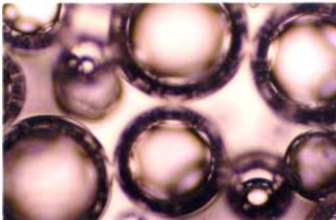
Fig. 3 – The gas-core aphrons can lump together, creating large aggregates and these macro-structures behave in the same manner as the individual aphron
