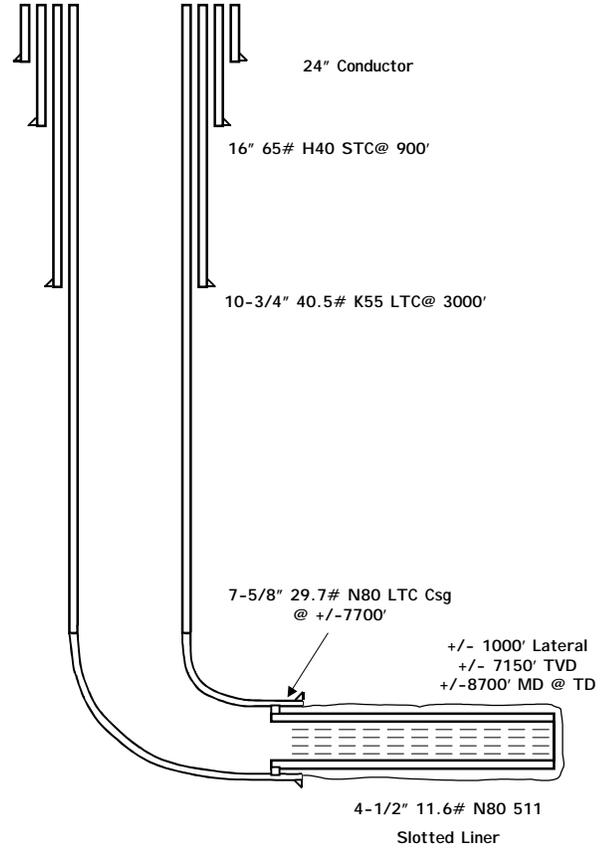
Fig. 8 – Typical Elk Hills well construction
