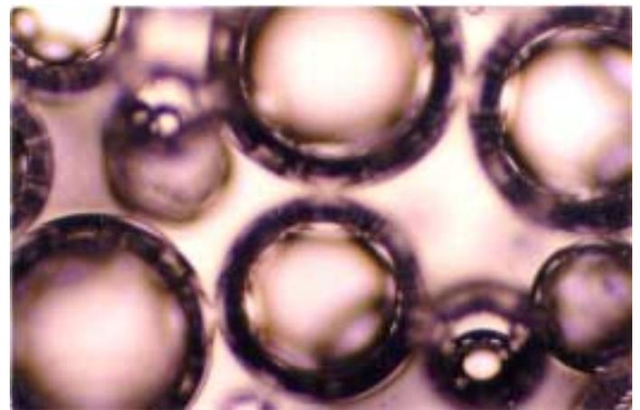
**Fig. 4** – Gas-core aphrons can clump together, creating large aggregates, and these macro-structures behave in a similar manner as an individual aphron.
