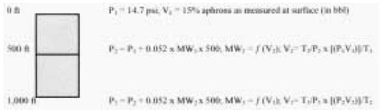
Fig. 6 – The Boyle's equation applied for 500-ft intervals to determine the aphron percentage, the interval-by-interval pressure and the corrected density.
