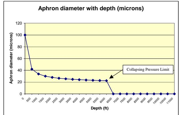
Fig. 8 – Aphron size change with pressure
