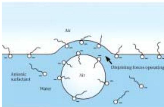
**Fig. 2** – Structure of a conventional surfactant-stabilized bubble<sup>2</sup>
