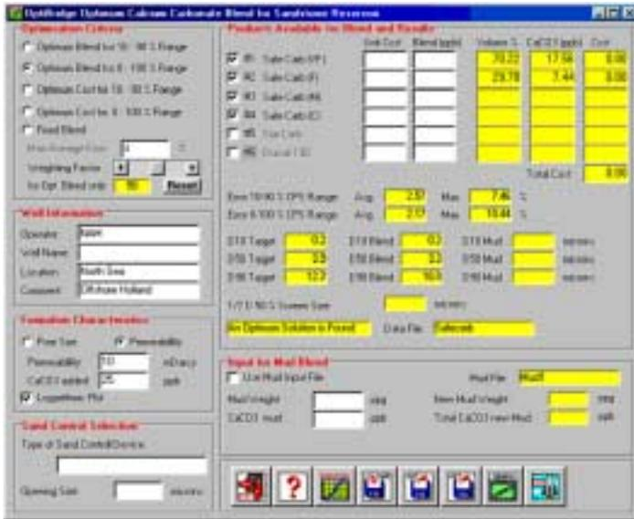
Fig. 5 – The optimum calcium carbonate blend based on the particle size distribution.
