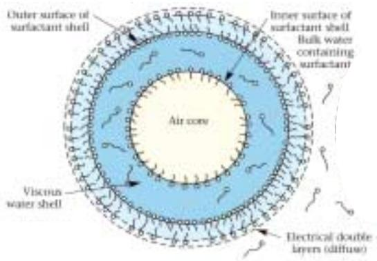
**Fig. 1** – Structure of colloidal gas aphron<sup>2</sup>
