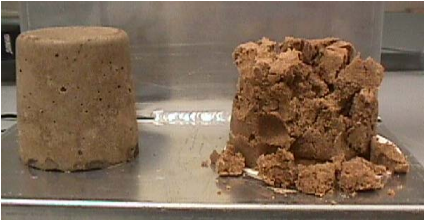
Figure 14 – Example of a loose sandstone core “solidified” using monomer material. The picture on the right shows a 6” sample of 500-600 mD sand before monomer treatment. Its compressive strength was only 20-30 psi and it allowed flow below a differential pressure of 100 psi. The figure on the left shows the same material after treatment, now with an elevated compressive strength of 140- 175 psi and a permeability of 0 mD with no flow through it at a differential pressure of 1500 psi N 2 gas.
