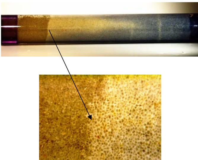
**Fig. 6 - Aphron Drilling Fluid Displays Bubbly Flow during Displacement of Water in 20/40 Sand**
