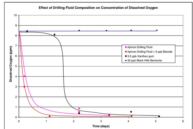
Fig. 4 - Oxygen in Aphron Drilling Fluids is Depleted Rapidly
