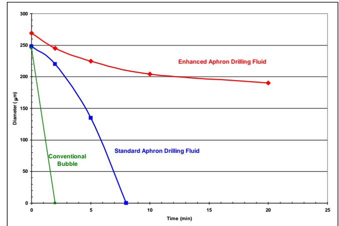
Fig. 3 – Longevity of Aphrons at Elevated Pressures is Much Greater than that of Conventional Bubbles 500 psig and Ambient Temperature
