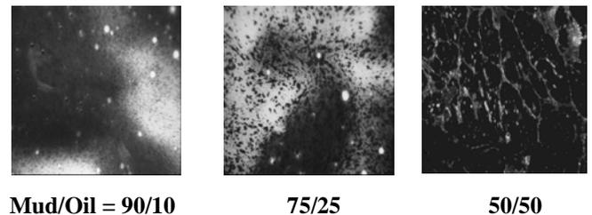
Fig. 15 - Aphron Drilling Fluid Mixes Readily with Canadian Crude Oil and is Water-Continuous up to at Least 25 vol % Oil
