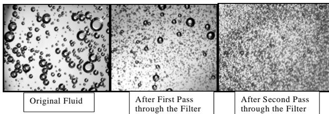
**Fig. 9 – Bubble Size Distribution in Transparent Aphron Drilling Fluid Changes after Passage through 15- $\mu\text{m}$  Filter**
