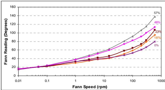
**Fig. 5 –Viscosity Profile of Aphron Drilling Fluids is not Greatly Affected by Presence of Small Amounts of Air**
