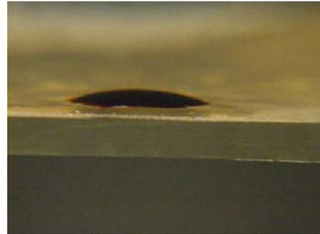
Fig. 14 - Crude Oil Nearly Spreads on Glass Surface Pre-Treated with Aphron Drilling Fluid
