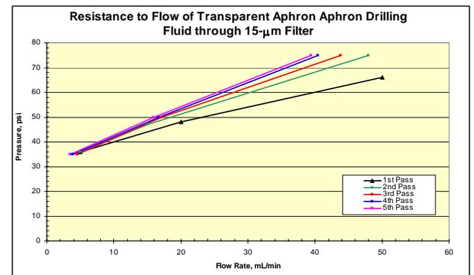
**Fig. 10 –Resistance to Flow in 15- $\mu\text{m}$  Filter of Transparent Aphron Drilling Fluid Increases after Multiple Passes through the Same Filter**
