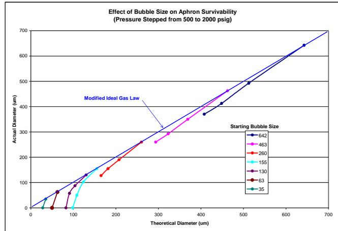
Fig. 2 – Aphron Longevity at Elevated Pressures Depends on Size
