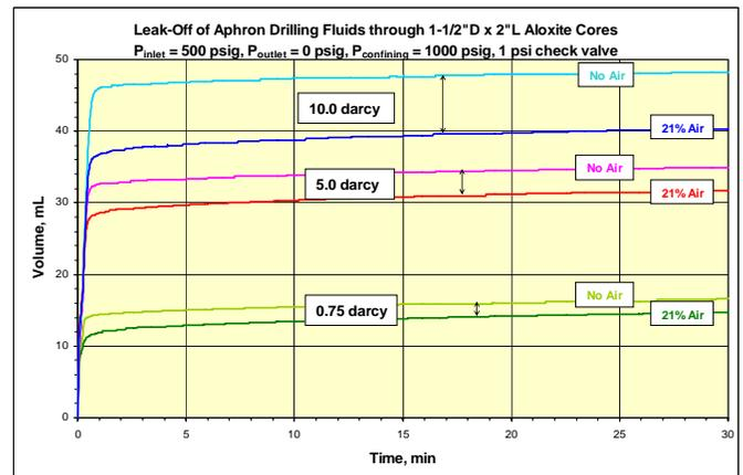
**Fig. 7 - Aphron Drilling Fluids can Seal High-Permeability Formations**
