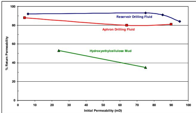
Fig. 12 - Return Permeability of Aphron Drilling Fluids is similar to that of Reservoir Drilling Fluids
