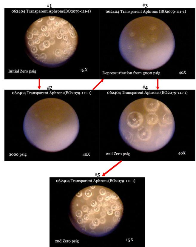
**Fig. 1 – Rapid Pressure Cycling of Aphron Drilling Fluids Leaves Most Aphrons Intact (Note that photos #2 - #4 are at higher magnification)**
