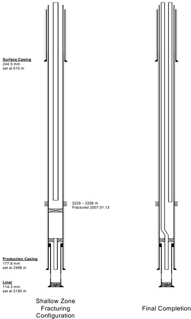
Fig. 1–Case 1: the shallow completion interval was killed using an oil based version of Aphron fluid technology in order to install a dead leg tubing string for hydraulic fracturing and then to configure well for dual string production.
