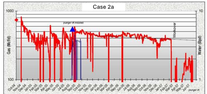
Fig. 6–Well production pre- and post-workover.
