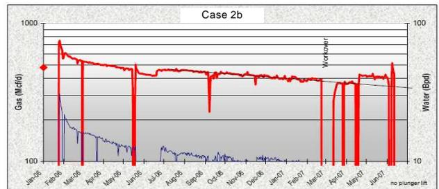
Fig. 9–Well production pre- and post-workover.
