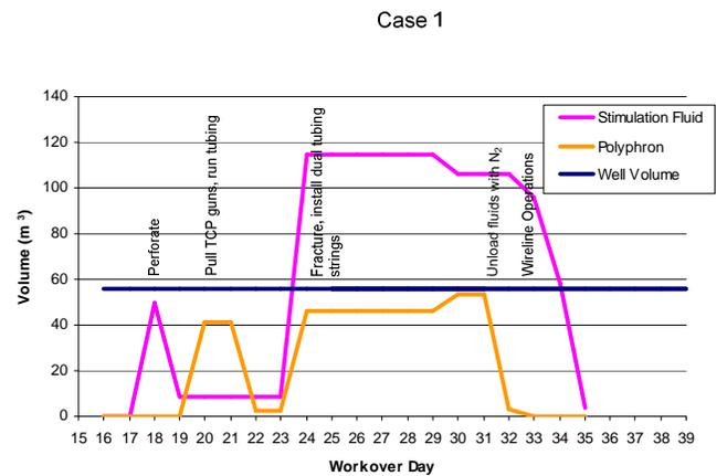
Fig. 3–Fluid losses are presented by fluid type with the major phases of the completion operation noted.
