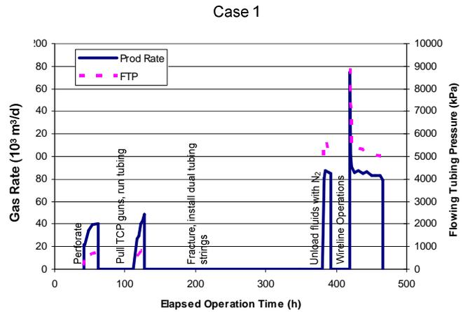
Fig. 2–Gas production rates observed during the completion operations.
