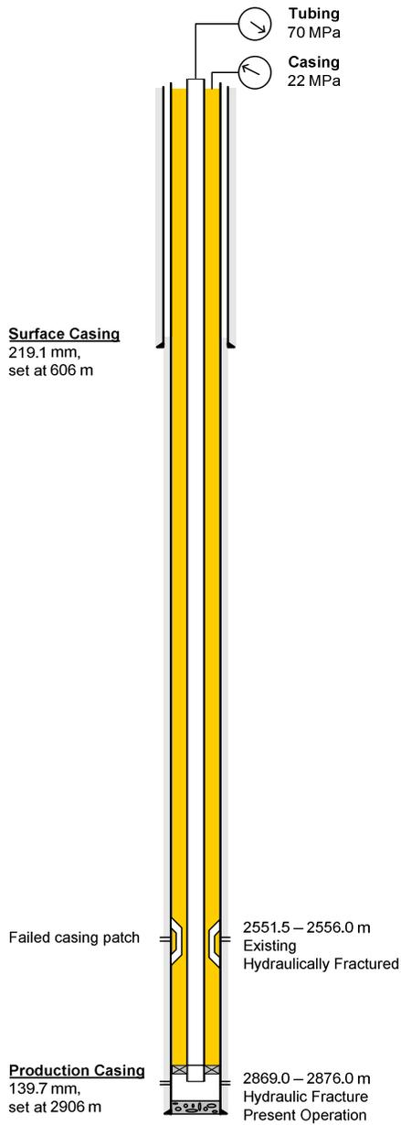
Fig. 10—Case 3a: a single zone was perforated and fractured below an existing hydraulically fractured completion interval. Aphron workover fluid was used to support a high annulus pressure after a temporary casing patch twice failed to set across the shallower interval.
