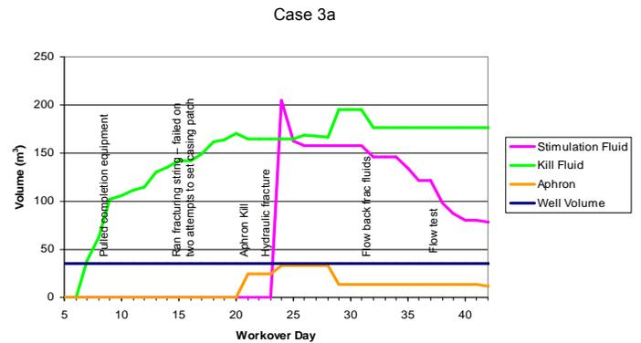
Fig. 11—Workover fluid losses are shown for each fluid type. High losses were incurred until the well was circulated over to an Aphron workover fluid on day 20.
