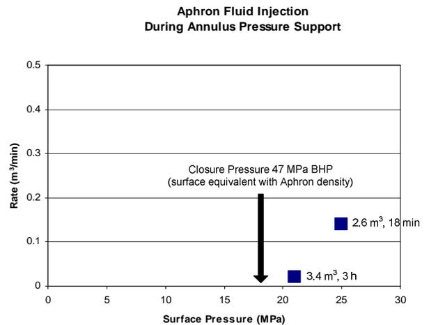
Fig. 12—Case 3b: annulus injection pressure observations suggest that the Aphron fluid provided an effective seal, even above the previously observed fracturing pressure of the upper interval. Injection volumes and durations are noted.
