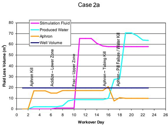
Fig. 5–Fluid losses are noted for each fluid type during the workover operations.
