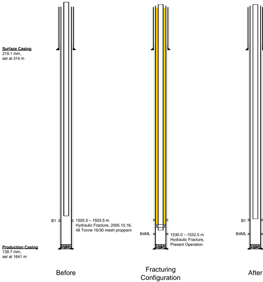
Fig. 7–Case 2b: a single zone was added and hydraulically fractured below an existing completion.
