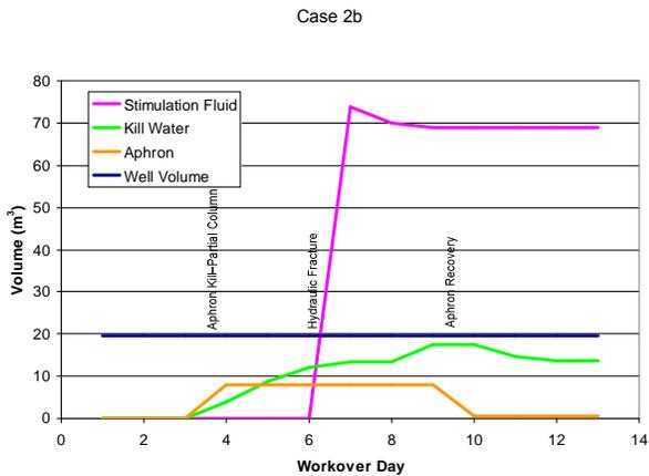
Fig. 8–Fluid losses are noted by fluid type during the workover operations. A partial column of Aphron workover fluid was used to kill the well. All Aphron fluid was recovered from the well during this operation.
