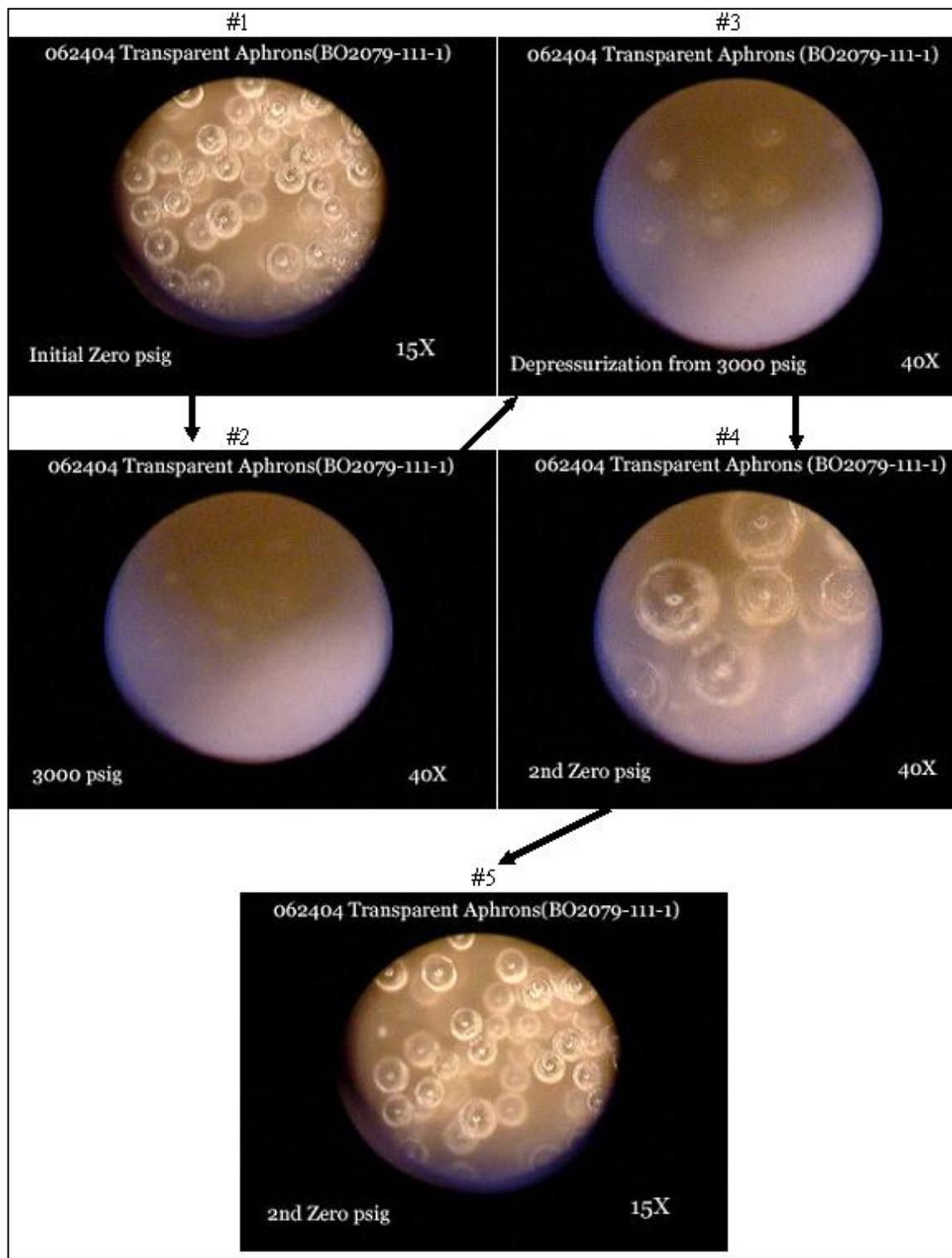
Large aphrons (> 100  $\mu\text{m}$  diameter) appear to be able to survive much better than small aphrons. Figure 2 shows the effect of the size of an aphron on its survivability.
