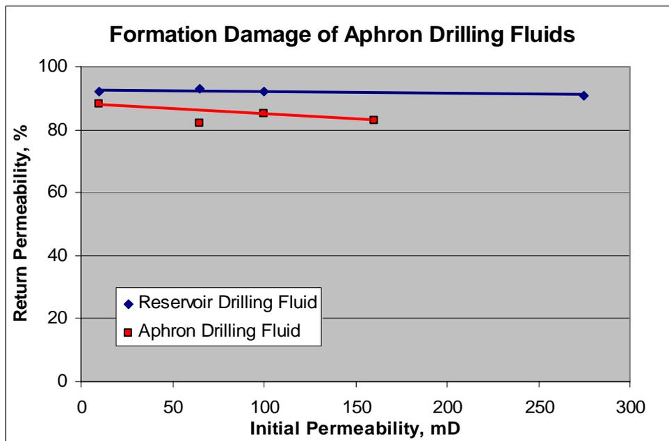
Finally, static linear leak-off tests demonstrate that aphron drilling fluids are capable of sealing rock as permeable as 80 Darcy. Figure 7 shows some data for aphron drilling fluids in synthetic Aloxite cores with permeabilities of 0.75 to 10 Darcy. It is clear that the base fluid itself is primarily responsible for slowing or halting loss of the drilling fluid, but properly designed aphrons may reduce these losses even further.
